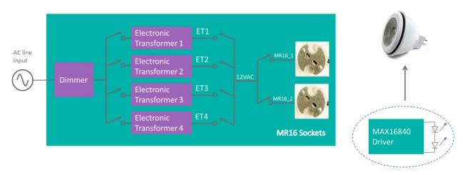
The demo includes a set of four electronic transformers which convert the line voltage to the 12V required by the MR16 bulb. A trailing edge dimmer precedes the electronic transformers and is used to turn the bulbs on and off and to dim the bulbs.
